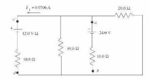
$$\begin{split} V_d + I_1 (10.0 \ \Omega) + 12.0 \ \mathrm{V} = V_c \\ V_c - V_d = 12.706 \ \mathrm{V}; \quad V_a - V_b = V_c - V_d = 12.7 \ \mathrm{V} \end{split}$$
